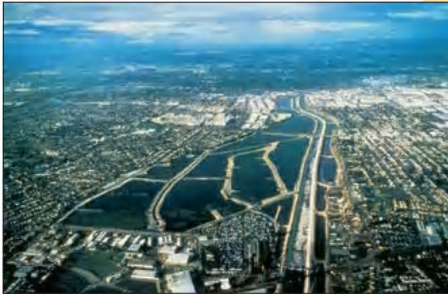
The Rio Hondo spreading grounds in California cover about 570 acres. Water for recharge is fed to the 20 shallow basins over a period of seven days. The basins are then drained for seven days and dried for an additional seven days.
